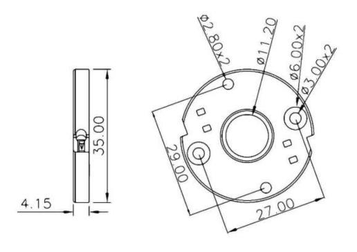
Chip-on-Board (COB) LED Array Holders: CREE LED LED Family: Cree>CXA1507, CXA1512, CXA1520
